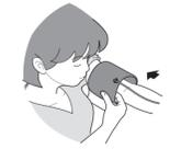
The bottom edge of the arm cuff should be 1 to 2 cm above the elbow. Marker (arrow under the air tube) is centred on the middle of your inner arm.
